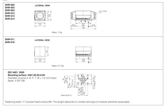
7 INSTALLATION DIMENSIONS OF SKR-0 VALVES [mm]
